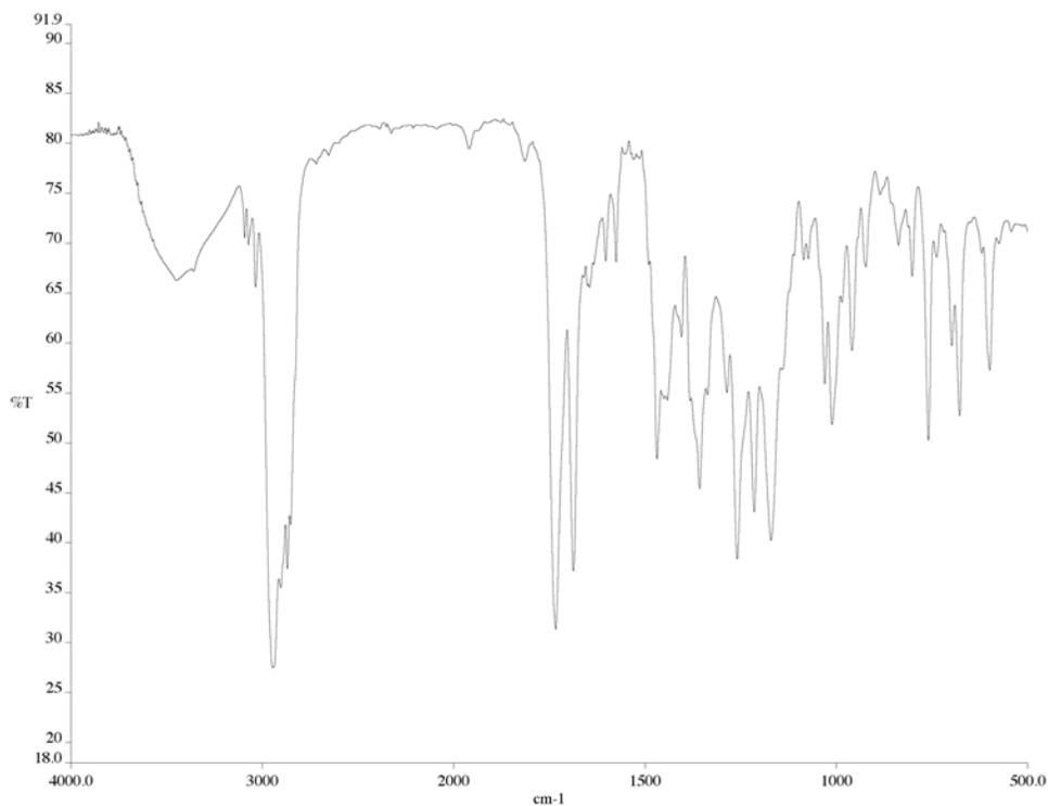
Figure A5.29 Infrared spectrum (thin film/NaCl) of compound **175h**.
