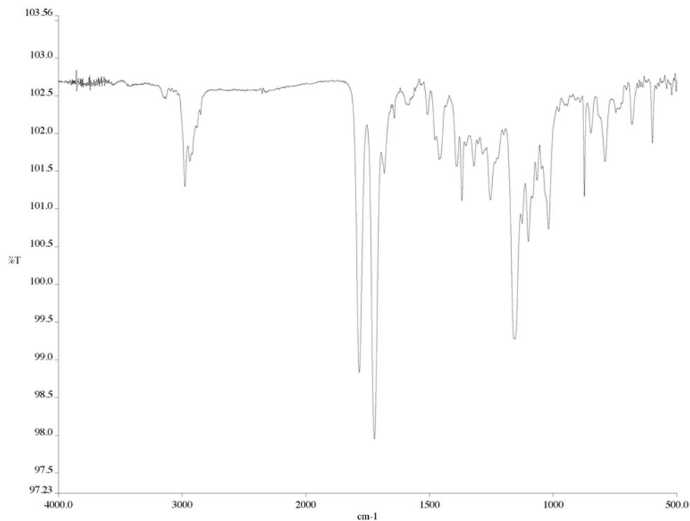
Figure A2.32 Infrared spectrum (thin film/NaCl) of compound **66b**.
