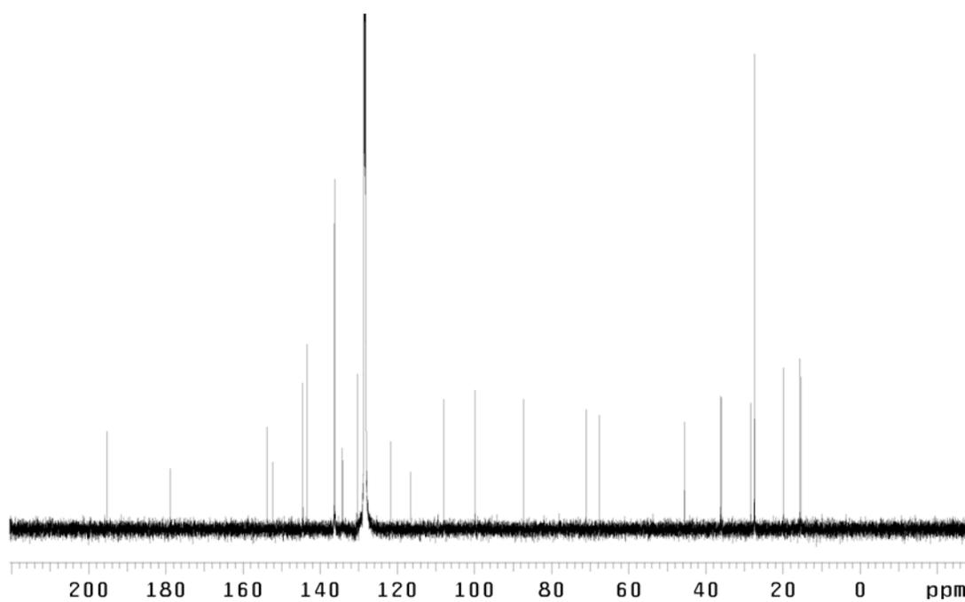
Figure A2.66 <sup>13</sup>C NMR (125 MHz, C<sub>6</sub>D<sub>6</sub>) of compound **71b(1)**.
