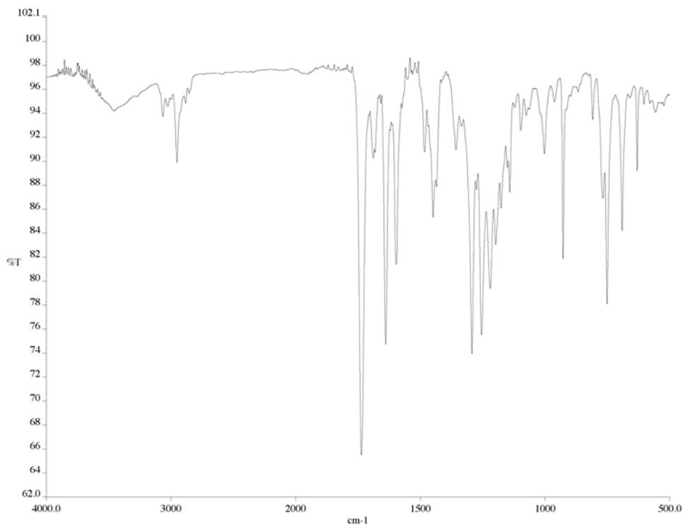
Figure A5.62 Infrared spectrum (thin film/NaCl) of compound **185d**.
