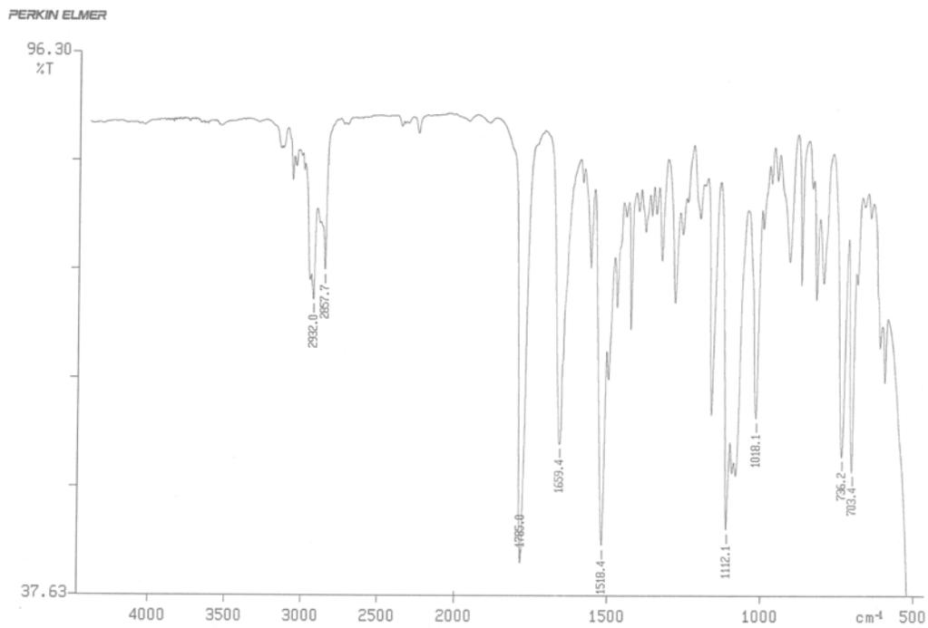
Figure A2.62 Infrared spectrum (thin film/NaCl) of compound **71a**.
