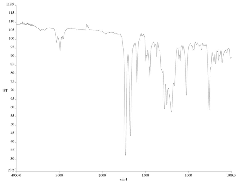
Figure A7.2 Infrared spectrum (thin film/NaCl) of compound **208**.
