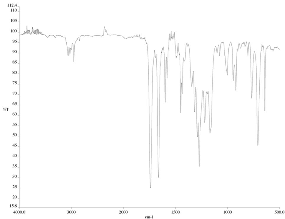
Figure A5.23 Infrared spectrum (thin film/NaCl) of compound **175f**.
