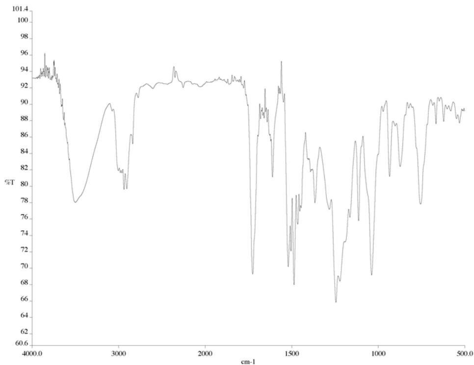
Figure A7.32 Infrared spectrum (thin film/NaCl) of compound **224**.
