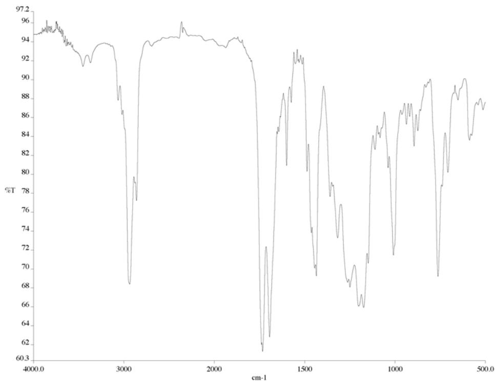
Figure A5.65 Infrared spectrum (thin film/NaCl) of compound **185e**.
