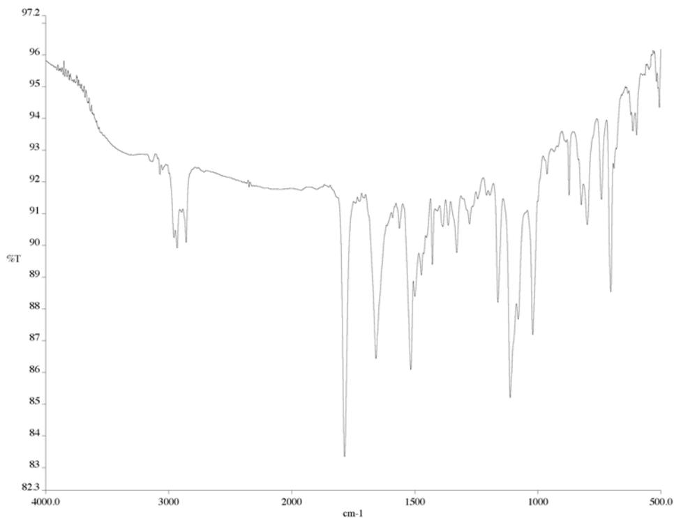
Figure A2.68 Infrared spectrum (thin film/NaCl) of compound **71b(2)**.
