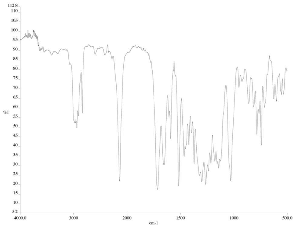
Figure A7.14 Infrared spectrum (thin film/NaCl) of compound **203**.
