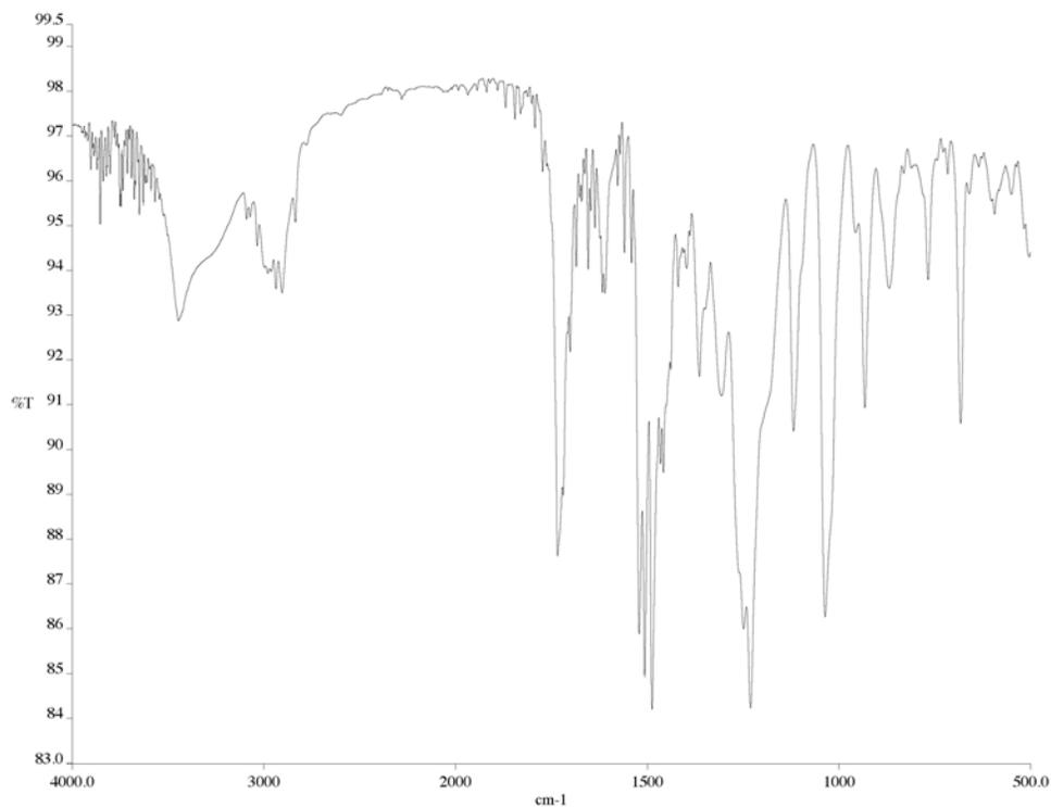
Figure A7.23 Infrared spectrum (thin film/NaCl) of compound **213**.
