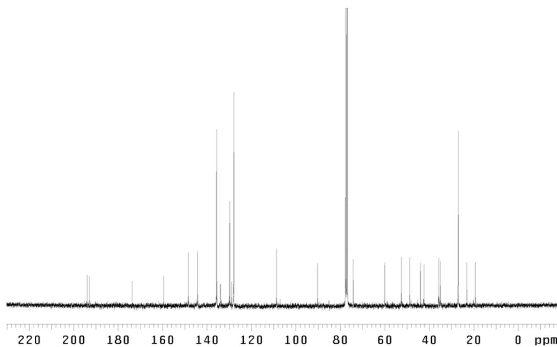
Figure A2.78 <sup>13</sup>C NMR (125 MHz, CDCl<sub>3</sub>) of compound **89**.
