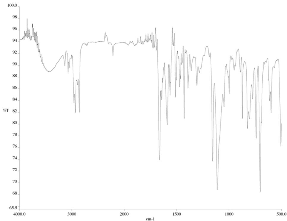
Figure A2.56 Infrared spectrum (thin film/NaCl) of compound **76**.
