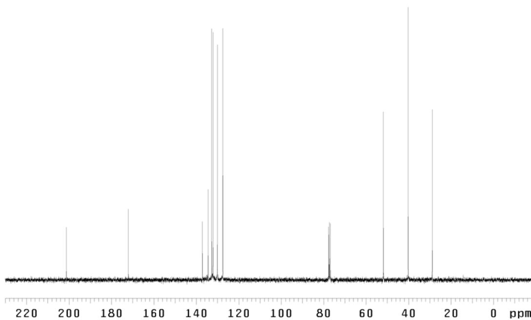
Figure A5.9 <sup>13</sup>C NMR (75 MHz, CDCl<sub>3</sub>) of compound **175a**.
