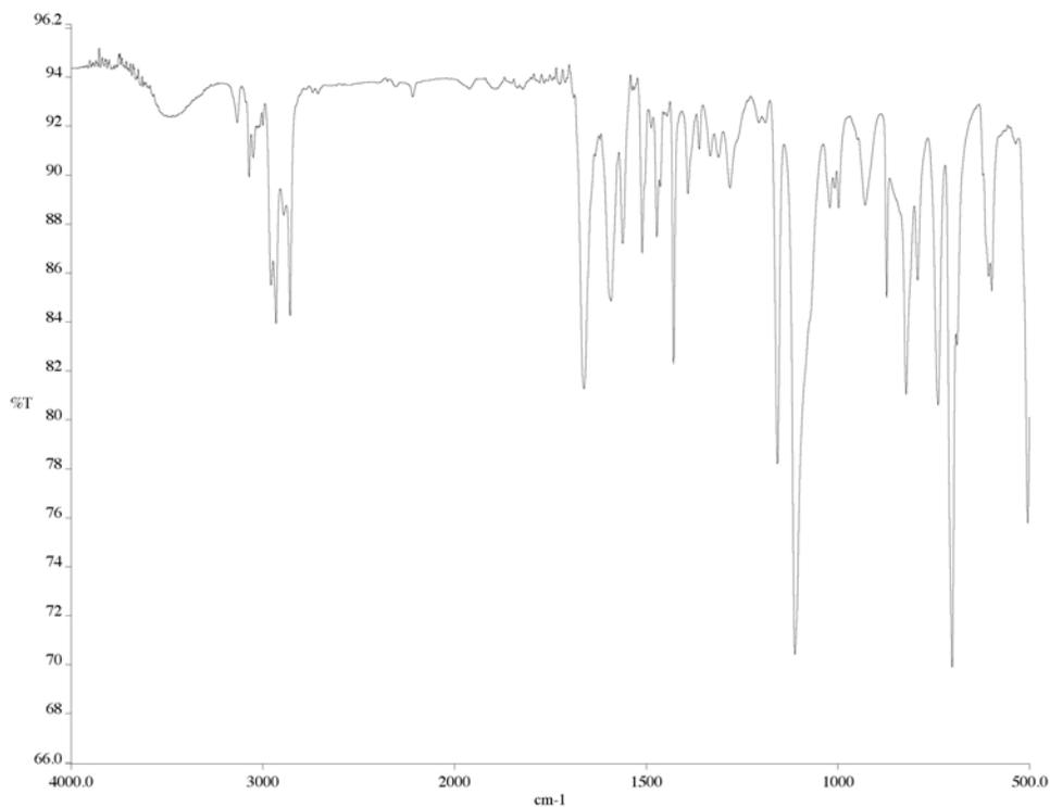
Figure A2.53 Infrared spectrum (thin film/NaCl) of compound **75**.
