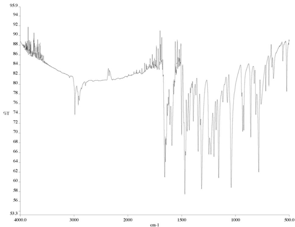
Figure A7.11 Infrared spectrum (thin film/NaCl) of compound **201**.
