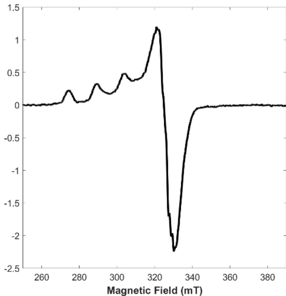
**Figure S3.** 77 K EPR Spectrum of **L8**•CuCl<sub>2</sub> in 2-MeTHF.
